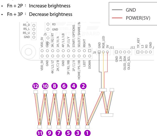
\*The order in which the RGB lights on the buttons illuminate will follow the wiring sequence. For example, the first connection will be numbered as 1, and so on.
