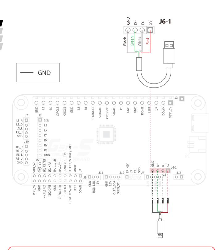
\* Please double-check whether the corresponding pin order is correct. Improper connection may cause the fighting board to burn.
