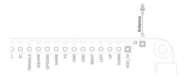
It is recommended to install the antenna to enhance stability during wireless gameplay.
